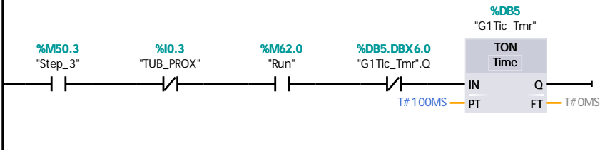
Network 6: Step 3 - Counter for retentive timer holding gate 1 open
